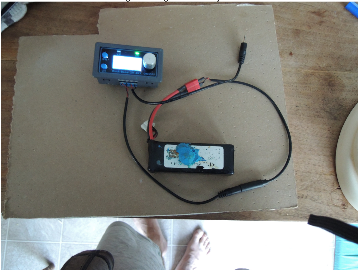
You can't see it in this shot, but the output voltage has been set to 3.22V. That's the voltage the unit will charge the supercapacitor to. It'll take a couple of minutes. The charging doesn't
